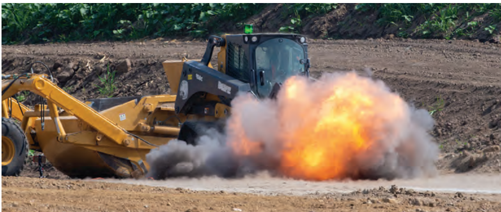
Above: On the Foundation's farm in Decatur, Illinois, an area has been set aside to test machinery for adaptation and survivability for use in demining in Ukraine. This 333G has been fitted with a forestry attachment which mimics a demining tool. It shows no damage after multiple blasts of 300 grams of the explosive material C4; the 300 grams exceeds the normal explosive material in an anti-personnel mine that would be found in Ukraine. Right: Inside the cab of a D-6 Cat bulldozer, equipment has been installed using John Deere Precision Agriculture Management System (AMS) accessories to provide mapping and driving capabilities for potential use in verifying Ukrainian farm fields are free of landmines. This tool also allows the vehicle to operate in a straight line, document the area covered, and is capable of operating a machine 24-hours a day. The Foundation is working to combine technology commonly used in agriculture and construction with equipment adapted to support demining in order to safely and more efficiently clear agricultural fields and bring them back into production.
